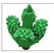
**Cutting Structure** The hole opener always have multi-cones. Bit cones are splited from Tricone Bitss and welded to bulid a big diameter bit. The pilot is attached with hole opener.
