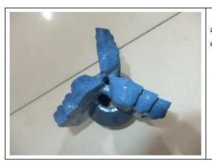
For drilling in soft formations, three or four-wing drag bits are available with either stepped or chevron profiles. Also available in certain sizes are replaceable wing drag bits
